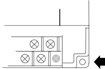
1.1 to 1.4Nm (10 to 12 in/lbs) of torque should be applied to M4 (#8-32) steel screws threaded into material containing internal threads and having a minimum thickness of 2.4mm (0.093in).
