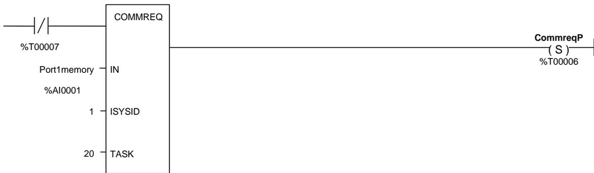
The following rung sets the bit COMMREQ Complete (%T7), which keeps the COMMREQ from being issued more than once and keeps the status from being overwritten.
