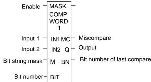
When the function receives power flow, it begins comparing the bits in the first string with the corresponding bits in the second string. Comparison continues until a miss-compare is found or until the end of the string is reached.
