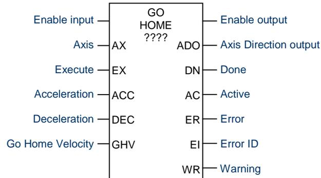
The channel's Output Enable bit (for example, Q0505 for channel 1) must be set to 1 to use this or any other motion function block. If the Output Enable bit is not 1, the function will not execute, and a Channel Enable error will be reported.
