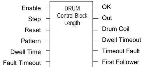
Power flow to the Enable input causes the Drum Sequencer to copy the content of a selected reference to the Out reference.
