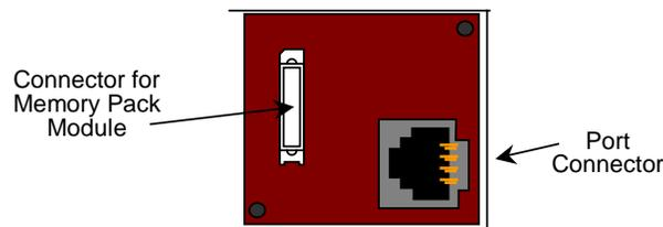
5. If a Memory Pack Module is being installed, orient the connector on the back of the Memory Pack Module with the connector on the Micro PLC or port-type Option Module. Press the Memory Pack Module downward until it clicks into place.
