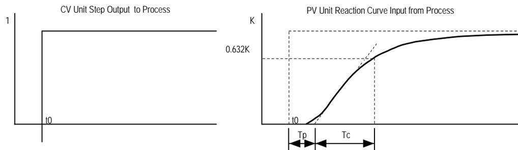
The following process model parameters can be determined from the PV unit reaction curve:
