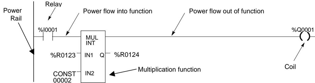
The flow of logical power through each rung is controlled by a set of simple program functions that work like mechanical relays and output coils. Whether or not a relay passes logical power flow along the rung depends on the content of a memory location with which the relay has been associated in the program. For instance, a relay might pass power flow if its associated memory location contained the value 1. The same relay would not pass power flow if the memory location contained the value 0.
