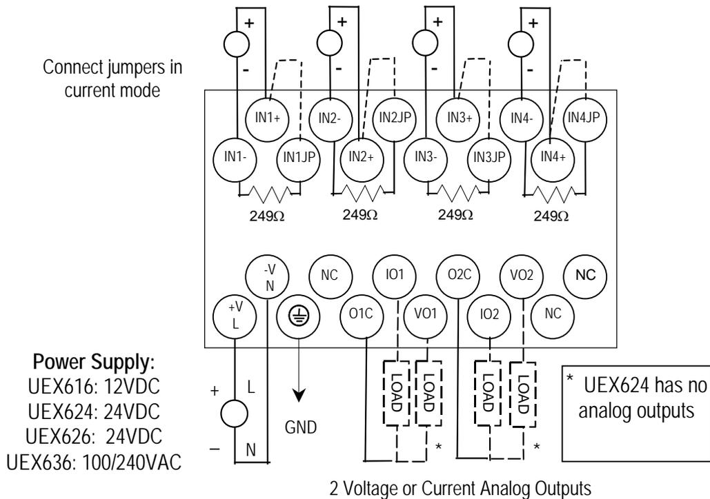
On modules IC200UEX616, UEX626 and UEX 636, voltage and current outputs are present on their respective output terminals at the same time. For proper module operation, only the output terminals that correspond to the voltage / current output configuration should be connected.
