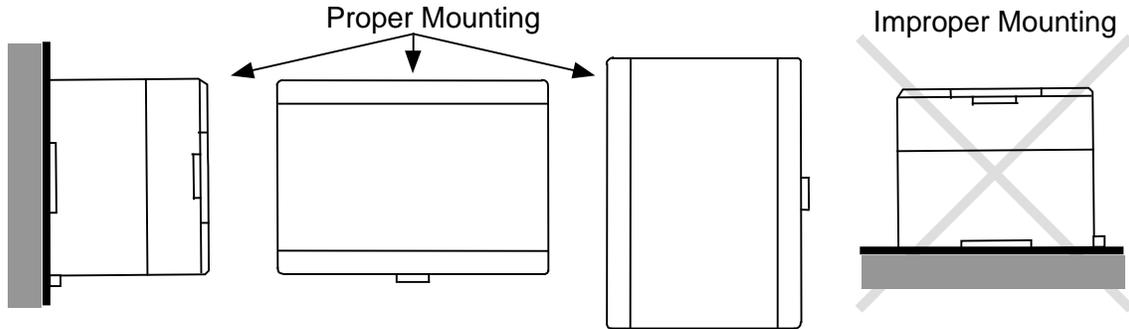
The DIN rail must be electrically grounded to provide EMC protection as described on the next page. DIN rails compliant with DIN EN50032 are preferred.
