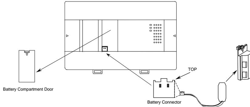
**For a cylinder-type battery**, tuck in the wires and snap the battery holder (see the illustration above) onto the VersaMax Micro PLC. The original battery compartment door is no longer needed.
