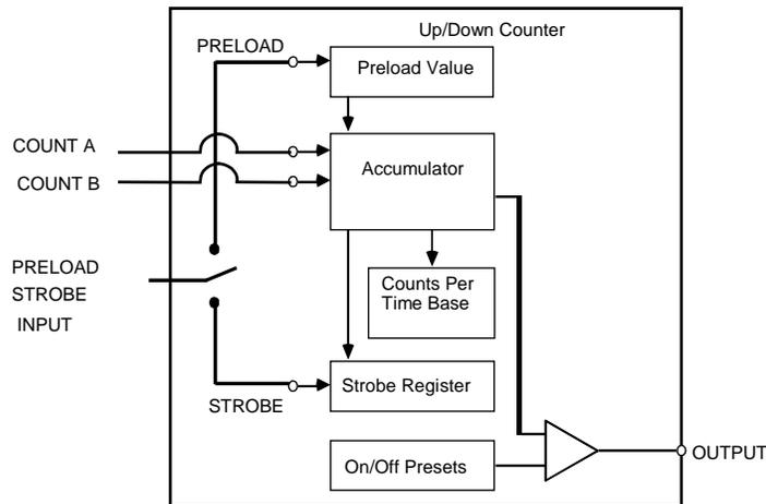
The counter counts continuously within its limits. The Accumulator wraps when the count limit is reached and continues counting. For example, if the Count Direction is up, when the count exceeds the High Limit by 1, the Accumulator value wraps to the Low Limit.
