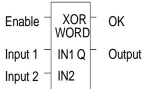
Each scan that power is received, the Exclusive OR function examines each bit in string IN1 and the corresponding bit in string IN2, beginning at the least significant bit in each. For each two bits examined, if only one is 1, then a 1 is placed in the corresponding location in bit string Q. The Exclusive OR function passes power flow to the right whenever power is received.
