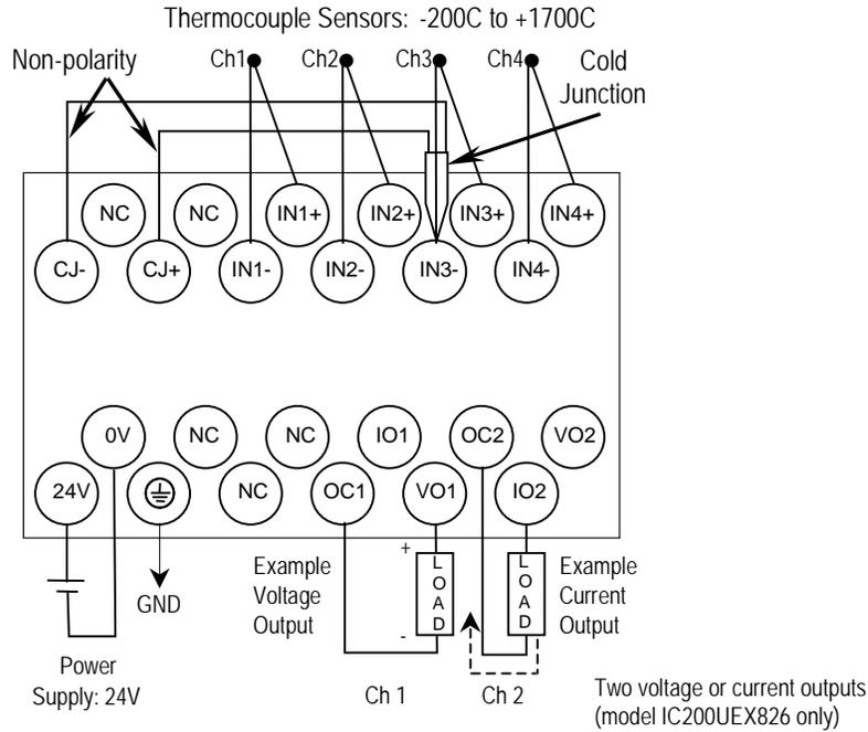
On module IC200UEX826, voltage and current outputs are present on their respective output terminals at the same time. For proper module operation, only the output terminals that correspond to the voltage / current output configuration should be connected.
