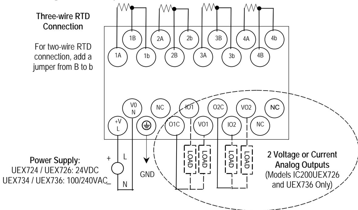
On modules IC200UEX726 and UEX736, voltage and current outputs are present on their respective output terminals at the same time. For proper module operation, only the output terminals that correspond to the voltage / current output configuration should be connected.
