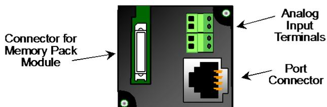
When installed on the Micro PLC, the RS-422/485 Port Option Module becomes port 2. It supports the following communications protocols:
