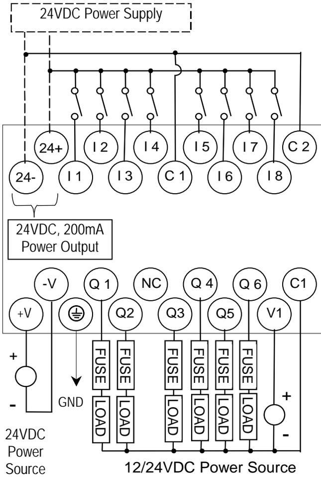
The maximum current that can be used for output points Q1 and Q2 is lower for ambient temperatures above 50°C.
