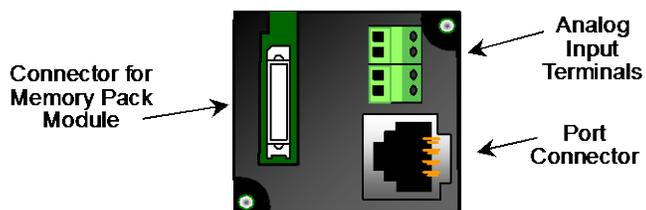
When installed on the Micro PLC, the RS232 Port Option Module becomes port 2. It supports the following communications protocols:
