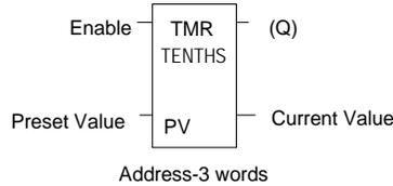
When the On-Delay Timer function receives power flow, the timer starts accumulating time (current value). The current value is updated when it is encountered in the logic to reflect the total elapsed time the timer has been enabled since it was last reset.
