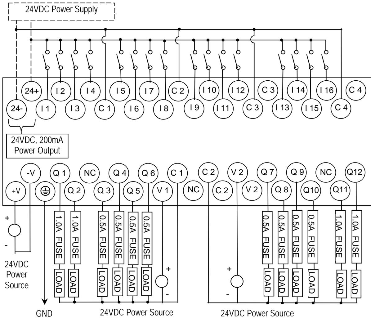
The maximum current that can be used for output points Q1, Q2, Q11 and Q12 is lower for ambient temperatures above 50°C
