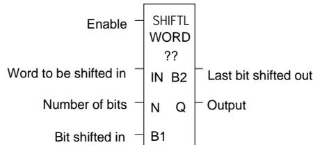
If the number of bits to be shifted (N) is greater than the number of bits in the array \* 16, the array (Q) is filled with copies of the input bit (B1), and the input bit is copied to the output power flow (B2). If the number of bits to be shifted is zero, then no shifting is performed; the input array is copied into the output array; and input bit (B1) is copied into the power flow.
