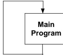
Or a program can be divided into subroutines. The maximum size of a main program block or subroutine block is 16K bytes. A Nano PLC application program can include up to 8 subroutine declarations. A Micro PLC application program can include up to 64 subroutine declarations. Subroutines can simplify programming and reduce the overall amount of logic. Each subroutine can be called as needed. The main program might serve primarily to sequence the subroutine blocks.
