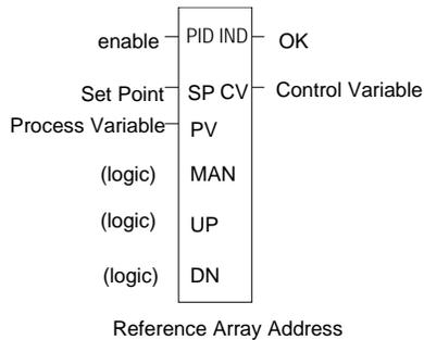
The PID function does not pass power flow if there is an error in the configurable parameters. It can be monitored using a temporary coil while modifying data.
