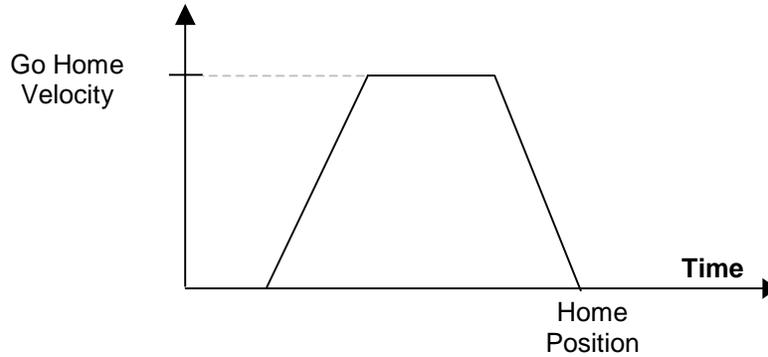
If a Home Offset was set up during execution of the Find Home function, the Go Home function causes the motor to move to the Home Offset position instead.
