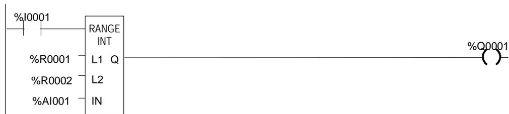
Output coil %Q0001 is On only if the value presently in %AI0001 is within the range 0 to 100.
