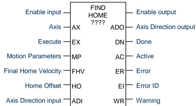
The channel's Output Enable bit (for example, Q0505 for channel 1) must be set to 1 to use this or any other motion function block on the channel. If the Output Enable bit is not 1, the function will not execute, and a Channel Enable error will be reported.
