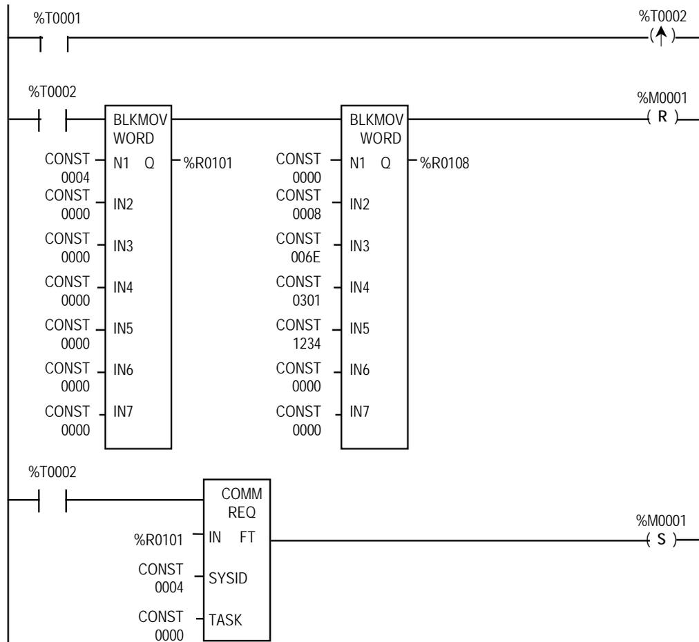
The first rung in the example includes a one-shot coil (%T0002) that executes the COMMREQ once. This prevents multiple messages from being sent.
