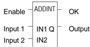
The standard math functions pass power if there is no math overflow. If an overflow occurs, the result is the largest value with the proper sign and no power flow.
