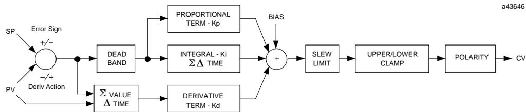
The ISA Algorithm (PIDISA) is similar except the  $K_p$  gain is factored out of  $K_i$  and  $K_d$  so that the integral gain is  $K_p * K_i$  and derivative gain is  $K_p * K_d$ . The Error sign, DerivAction and Polarity are set by bits in the Config Word user parameter.
