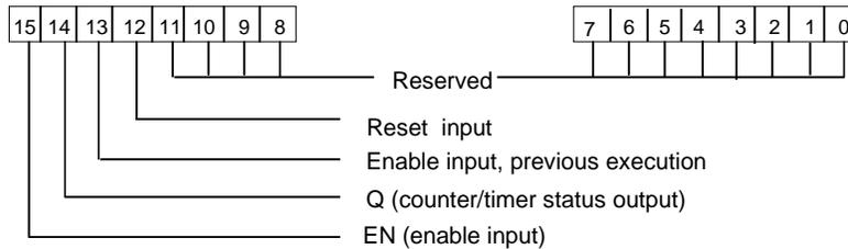
Bits 0 through 11 are used for timer accuracy; not for counters.
