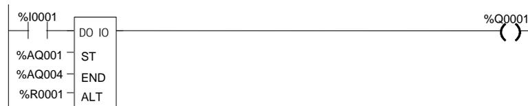
If no reference were specified for ALT, the PLC would write values at references %AQ001-004 to analog output channels.
