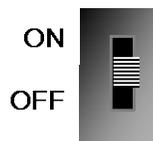
The Write Protect switch on the Memory Pack Module prevents writing data to the module when it is in the ON position.
