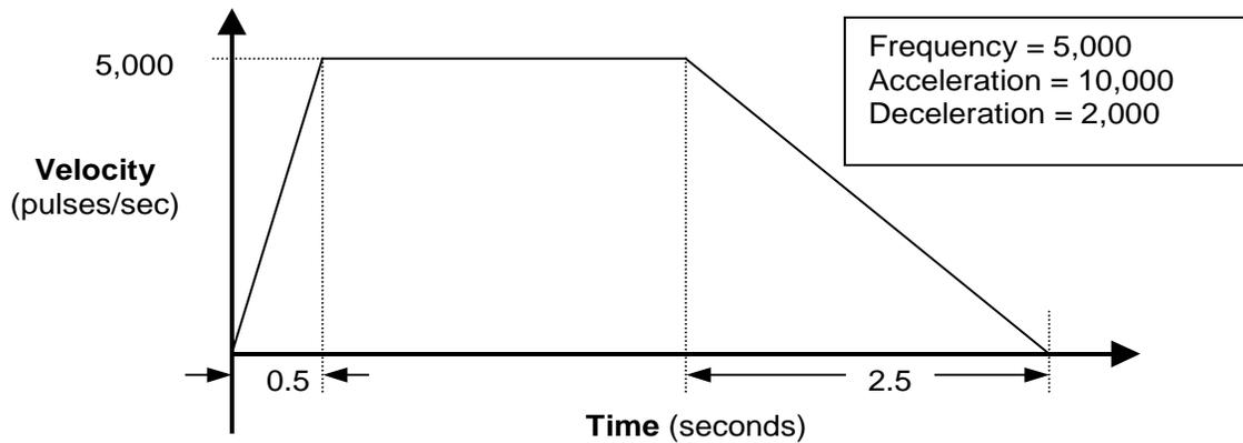
For the example above, the ramp up time is 500ms (1/2 second), so the ramp up takes place in 5 steps: 100ms, 200ms, 300ms, 400ms, 500ms with frequencies of 1kHz, 2kHz, 3kHz, 4kHz, and 5kHz respectively.
