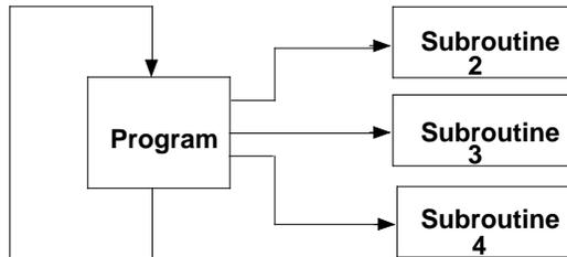
A subroutine block can be called many times as the program executes. Logic that should be repeated can be placed in a subroutine block, reducing total program size.
