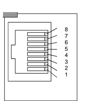
Note: There is no shield or frame-ground or shield pin on this connector.
