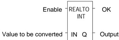
Note that loss of precision can occur when converting from Real-type data to Double-Precision Integer, because Real data has 24 significant bits.
