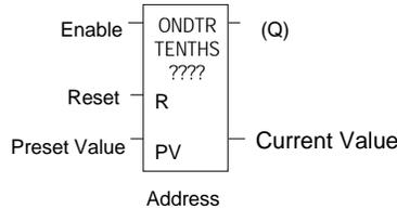
When the current value equals or exceeds the preset value PV, output Q is energized. As long as the timer continues to receive power flow, it continues accumulating until the maximum value is reached. Once the maximum value is reached, it is retained and output Q remains energized regardless of the state of the enable input.
