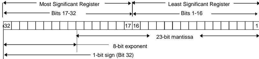
For example, if the floating-point number occupies registers %R0005 and %R0006, then %R0005 is the least significant register and %R0006 is the most significant register.
