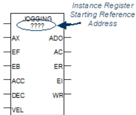
Each instance of a motion function block in the program requires a separate memory area for its internal status and control data. This must be set up by assigning two contiguous words of %R memory during programming. The reference address location is initially indicated by ??? in the function block.
