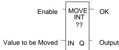
Note that if an array of Bit-type data specified in the Q parameter does not include all the bits in a byte, the transition bits associated with that byte (which are not in the array) are cleared when the Move function receives power flow.
