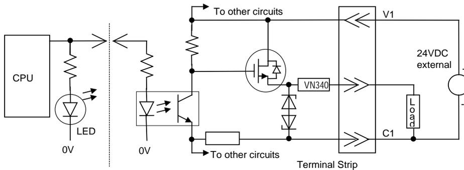
For Micro 10-, 14-, 23- and 28- PLCs, when using the outputs as PWM or Pulse Train Outputs, and for duty cycles in the lower ranges (5% and lower), a pulldown resistor must be connected between the output point (Q1-Q3) and the common terminal (C1). A 1.5 k $\Omega$ , 0.5 watt resistor is recommended.
