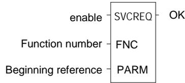
When the SVCREQ receives power flow, the PLC is requested to perform the function number (FNC) indicated. Parameters for the function are located beginning at the reference given for PARM. This is the beginning of the "parameter block" for the function. The number of 16-bit references required depends on the SVCREQ function being used.
