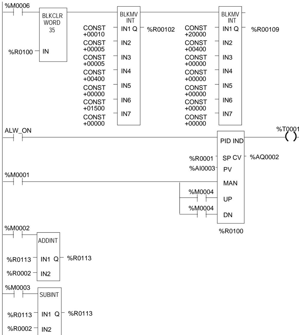
The block can be switched to Manual mode with %M1 so that the Manual Command, %R113, can be adjusted. Bits %M4 or %M5 can be used to increase or decrease %R113 and the PID CV and integrator by 1 every 100 ms solution. For faster manual operation, bits %M2 and %M3 can be used to add or subtract the value in %R2 to/from %R113 every PLC sweep. The %T1 output is on when the PID is OK.
