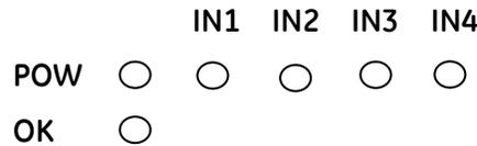
If an initialization error occurs, the OK LED blinks rapidly. During normal operation, the analog input LEDs should be off.
