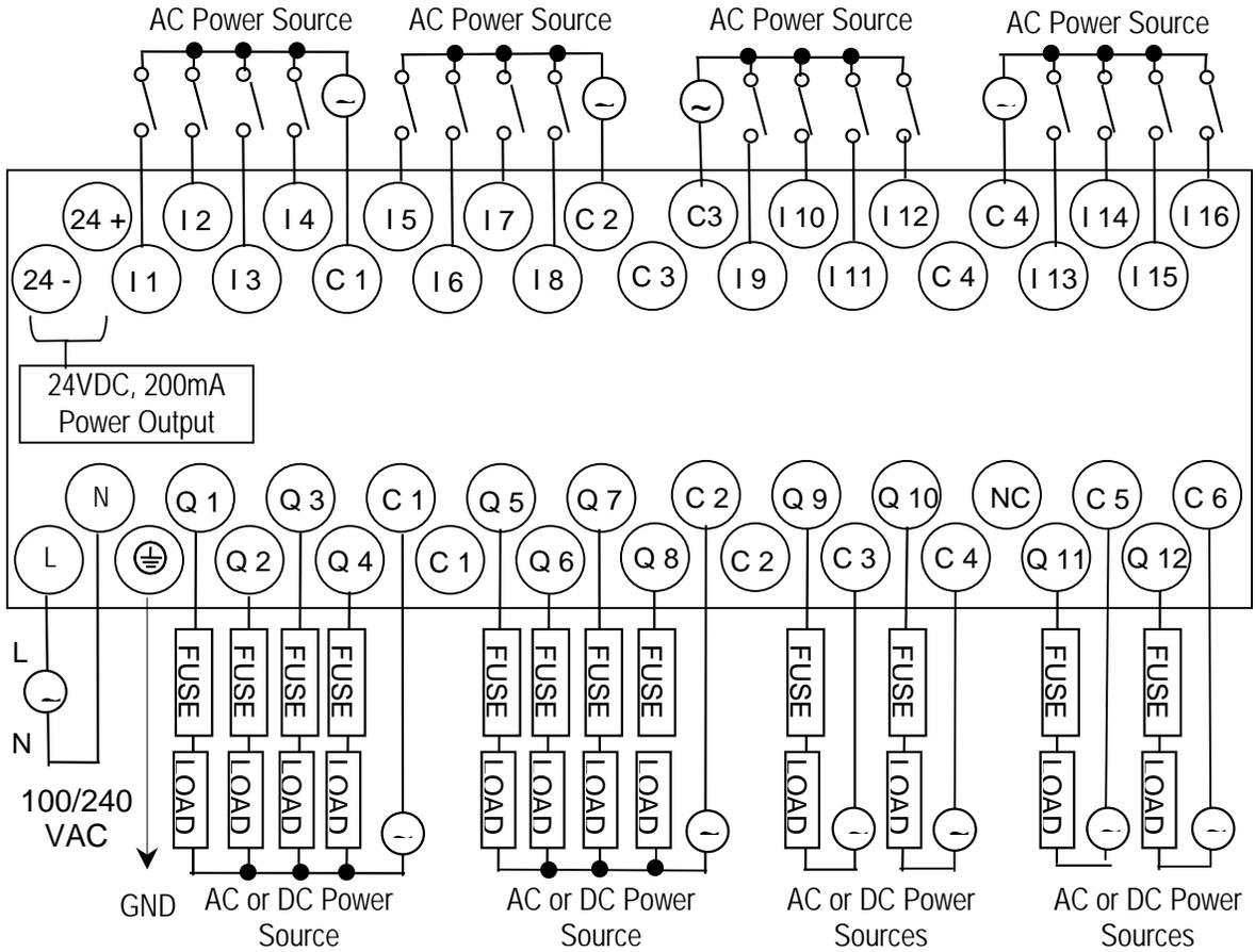
Outputs Q 1 – Q 10 are rated at 2.0 Amps each. Outputs Q 11 and Q 12 are rated at 10.0 Amps each.
