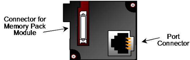
When installed on the PLC, the Ethernet Port Option Module becomes Port 2. It supports the following communications protocols:
