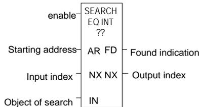
The search continues until the array element of the search object (IN) is found or until the end of the array is reached. If an array element is found, the Found Indication (FD) is set ON and the Output Index (output NX) is set to the relative position of this element within the array. If no array element is found before the end of the array is reached, the Found Indication (FD) is set OFF and the Output Index (output NX) is set to zero.
