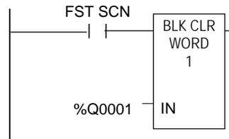
Other system status reference nicknames include T\_10MS, T\_100MS, T\_SEC, and T\_MIN (see below), FST\_SCN, ALW\_ON, and ALW\_OFF.
