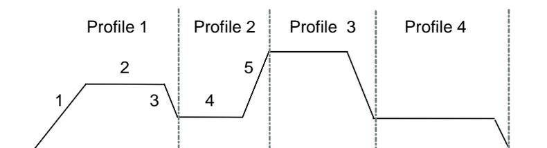
In this example, segments 1, 2, and 3 use the profile 1 parameters:
