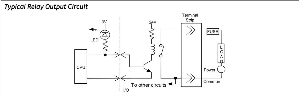
Installing suitable suppression across inductive loads enhances reliability of relay contacts. When switching inductive loads, relay contact life approaches resistive load contact life if suppression circuits are used. The 1A, 100V diode shown in the typical DC load suppression circuit is an industry standard 1N4934.
