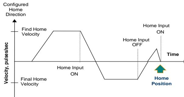
1. After accelerating to the configured Find Home Velocity, the axis moves in the specified direction until the Home Input signal is detected.
