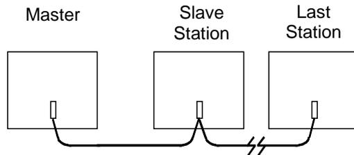
The RS-485 line must include handshaking and use wire type specified earlier. Reflections on the transmission line can be reduced by daisy-chaining the cable as shown. Make connections inside the connector to be attached to the PLC. Avoid using terminal strips to other types of connectors along the length of the transmission line.
