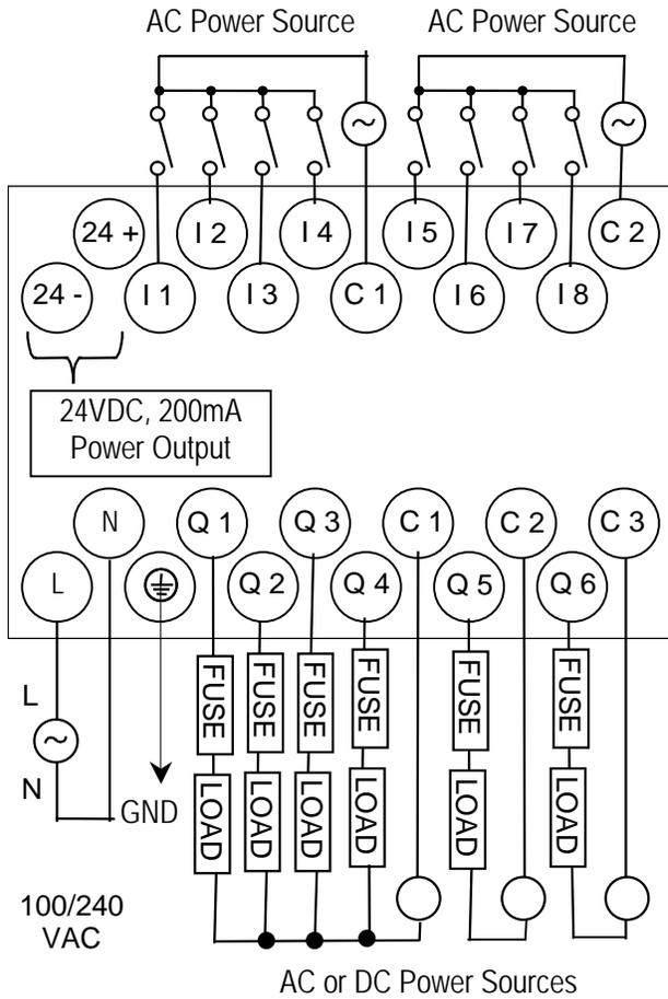
Outputs Q 1 – Q 4 are rated at 2.0 Amps each.
